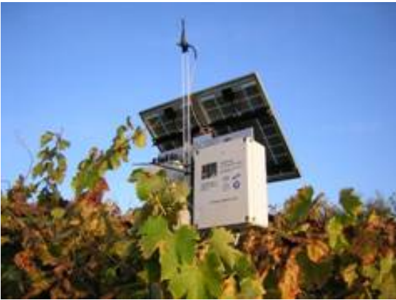
Figure 14: Aml node in the vineyard
