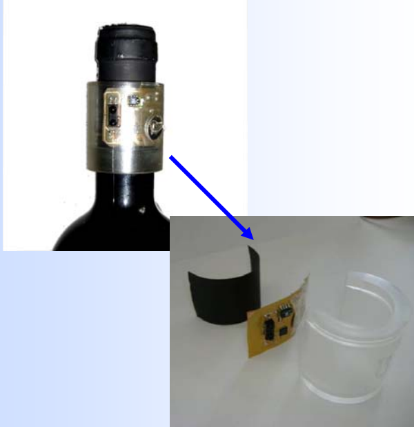
Figure 10: The smart tag integrated in the bottle of wine
