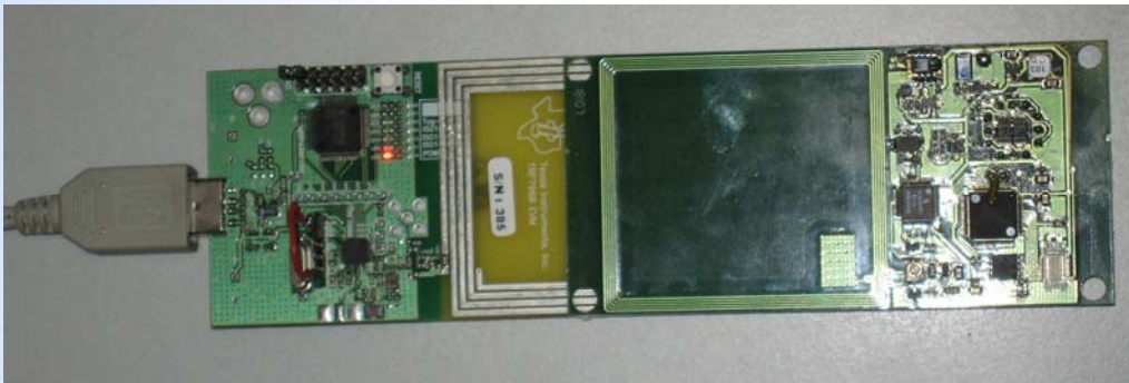
Figure 8: Tag prototype, developed on PCB substrate, together with the commercial TI reader used for this demonstration.
